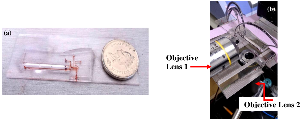
Figure 4. (a) Micro-chip and (b) the set up to visualize lateral and vertical position of the main flow. Objective lens 1 was used for lateral imaging and recording the flow pattern from side. The Objective lens 2 was used to vertically image the flow pattern from top.
