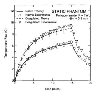
**Figure 4.** Temperature rise in polyacrylamide phantom with static optical properties. Thermocouple probe measurements at r = 5.3 mm with theoretical predictions for polyacrylamide phantom with the optical properties of native (lower curve) and coagulated (upper curve) albumen phantom. Error bars represent the error in numerical prediction based on uncertainty in thermal property value, fibre coupling efficiency and thermocouple positions.
