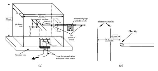
**Figure 3.** (*a*) Schematic diagram of apparatus used to measured the temperature rise within phantoms. (*b*) close-up of thermocouples and fibre tip.
